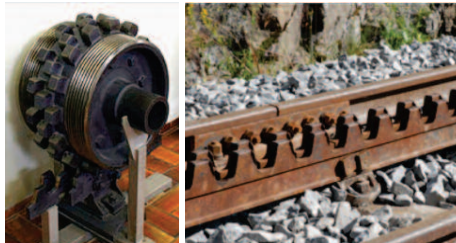
Abt; rack and pinion system used on the Furka railway
